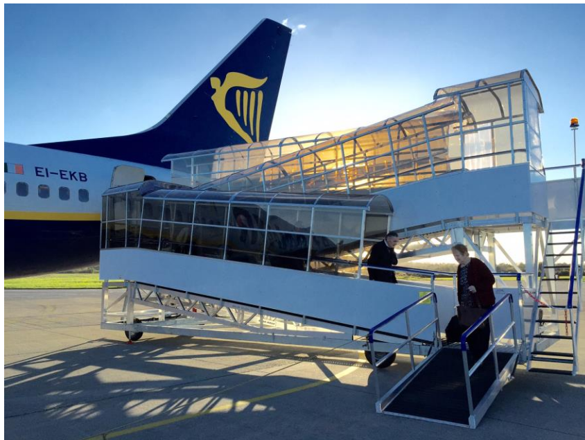
Figure 6-1. Accessible mobile boarding ramp, Kerry Airport, Ireland
